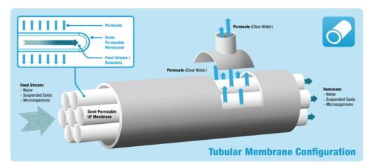
The tubular module design uses polymeric membranes cast on the inside of plastic or other components with diameters typically in the range of 5 - 25 mm with lengths from 5 - 20 ft.
